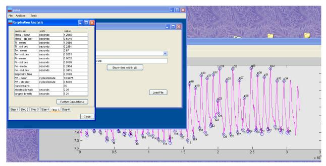
Figure 15. Appearance of puka at Step 5 of respiration signal analysis.
