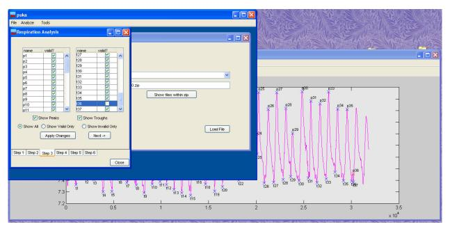
Figure 13. Appearance of puka during Step 3 of the respiration analysis. Trough t36 is unchecked so that it will not be included as a breath.
