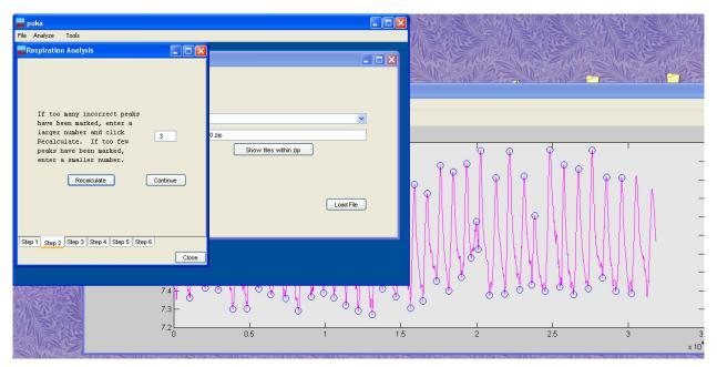
Figure 10. Respiration signal with the peaks and troughs correctly identified. The threshold was raised from 0.1 to 0.3.
