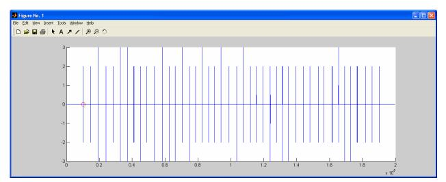
Figure 7. Onset trigger channel showing detected trigger location (circle).
