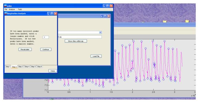
Figure 9. Step 2 of respiration analysis, in which the peak detection algorithm is used to identify the breaths. Too many points have been marked as "breaths," indicating that the threshold needs to be increased.
