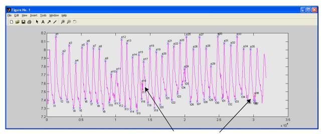
Figure 12. Respiration signal at the start of Step 3. p16, p36, and t17 were correctly marked (as invalid) for exclusion, but t36 was not.
